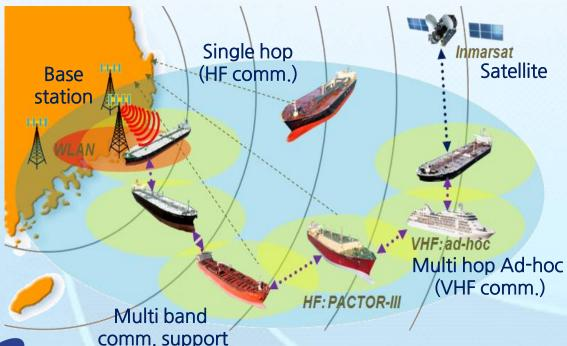
A research on the multi band ad-hoc technology that connects selectively to adequate channels, considering different circumstances, is in progress
