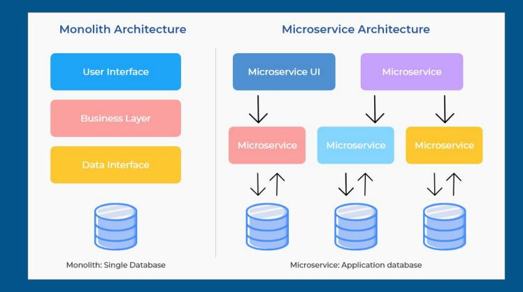
"the microservice architectural style is an approach to developing a single application as a suite of small services, each running in its own process and communicating with lightweight mechanisms, often an HTTP resource API."
