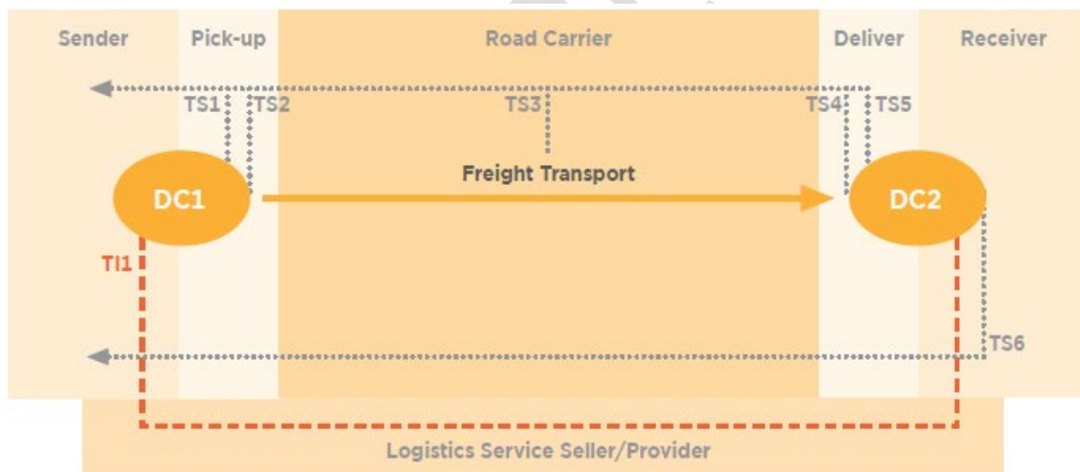
Figure 16. Typical TI and TS message exchanges involved for a single freight consignment; GS1 Australia, 2020 - Freight Data Exchange Pilot Project - Summary Report
